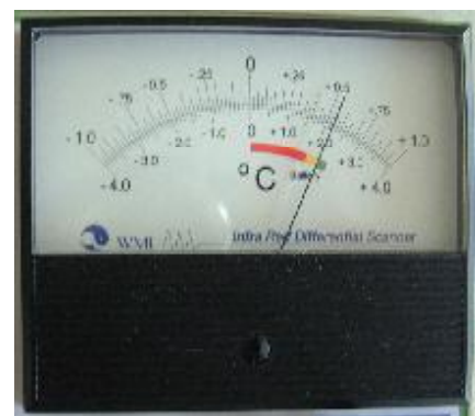
The meter showing a positive reading of +2.2 °C.
