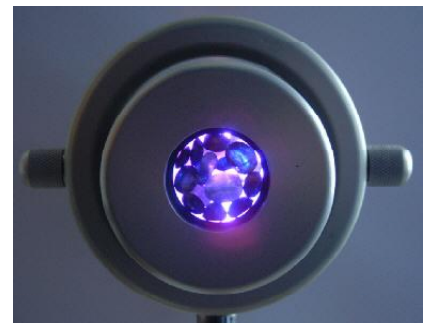
Lux IV Lamp Transducer fitted with a violet filter & filled dark sapphires.
