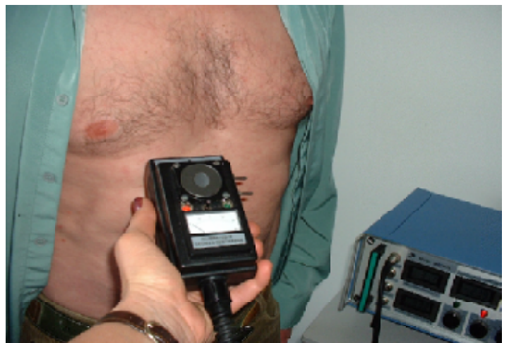
Fig 5. Scanning infrared emissions using an early prototype infrared scanner calibrated against platinum temperature references.
